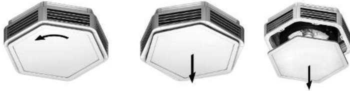
Fig. 32: Dismantling the housing cover
