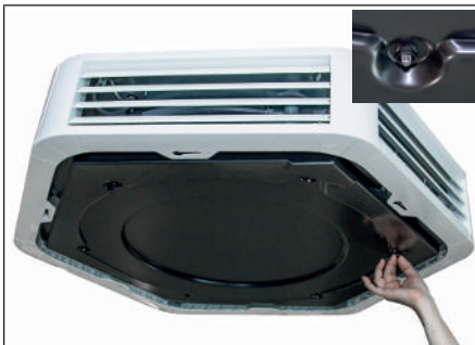
Fig. 33: Unscrewing the plug-in nut on the condensate tray
